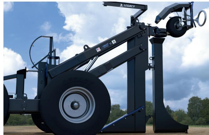
We recommend in most soil types and conditions when installing tile deeper than 48"-60" and larger than 8" drain tile that a "pre-rip pass" be made. The pre-rip pass will break up the hard soil deep below the surface and displace that large volume of soil that you need to move.
