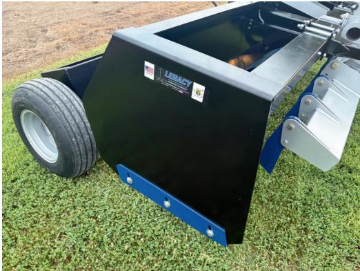
It can also be paired with any of our Laser or GPS Technology options to be a precise finish grader as well. With certain grade control options it can operate both Elevation and Tilt.
