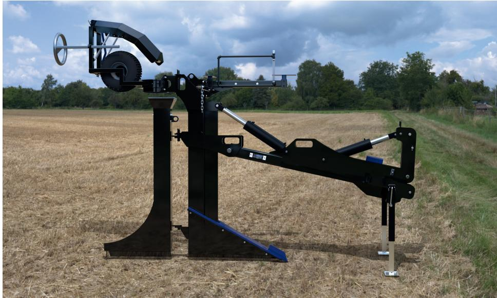
**Fork pockets in frame for easy handling when not hooked to a tractor**
